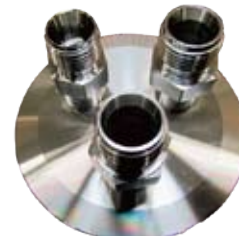
Welding of vacuum parts
