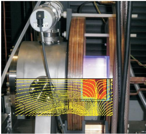
Figure 1: Picture of the experimental setup and the discharge, showing two regions with different optical emission. The lower half of the figure shows also the configuration of the magnetic field lines.
