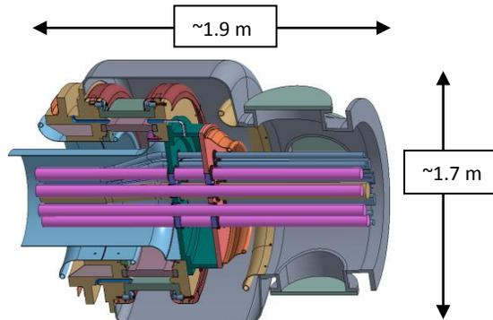
Figure 1 DNB High Voltage Bushing
