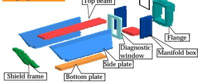
The upper port plug should has high stiffness since the port plug is cantilevered structure. To achieve such high stiffness, the upper port plug is designed to compose of forging material.
