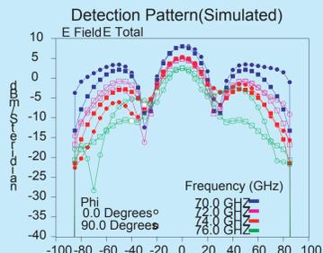
Axisymmetric pattern is realized with directivity of 5dBi.
