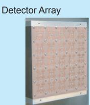
25 (5x5) detectors are arranged. IF outputs are introduced to back side of the substrate via microstrip line to coplanar line transformer.
