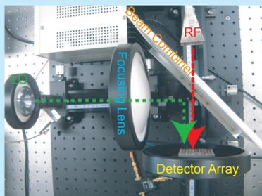
Instead of the dichroic plate utilized in preliminary experiment, the dielectric plate with a thickness of 400um and  $\epsilon=10.2$  is utilized as a beam combiner. Transmissivity and reflectivity of the plate are 0.5 and 0.5 around 70-80GHz, respectively
