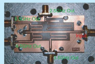
In order to achieve better performance and smaller size of the IF system, the power divider and the bandpass filters are replaced by the circuit as shown in left picture. The IF signal is coupled to each bandpass filter, which contributes better performance of the return loss at the input port. The video detectors have also been developed by the MIC technology to achieve higher sensitivity and lower cost.
