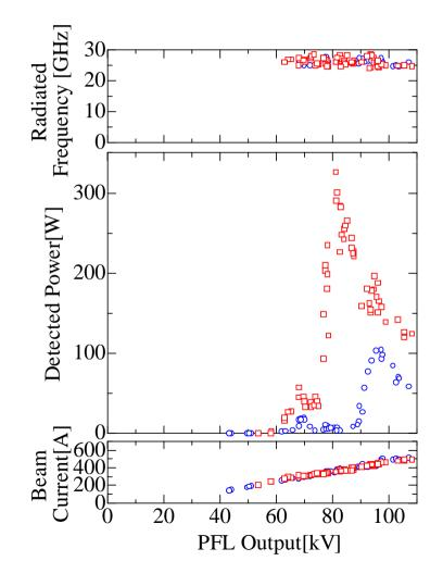
(□) for BWO with the Bragg refractor and (○) for BWO without the Bragg refractor.
