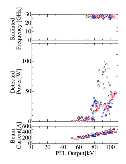
Beam input end is :(O) the 25.5 GHz SWS,( $\Delta$ ) 34 mm smooth waveguide terminated by mesh and ( $\diamond$ ) 68 mm smooth waveguide terminated by mesh.
