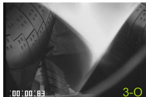
Transition of the bright area on the divertor legs from right to left side with the radial position of the magnetic axis ( $R_{ax}$ ) is observed from an outer port (3-O).
