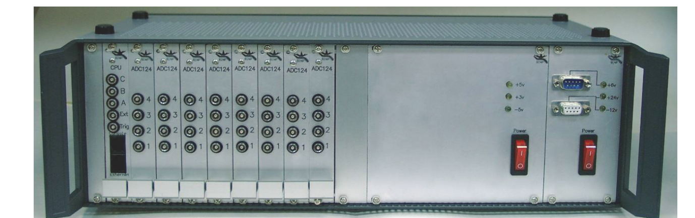
Fig.9. Synchronous 32-channel × 40 MS/s data acquisition system with multiplexer, TCP/IP Ethernet controller and power supply units. Each 12-bit ADC comprises 64 MB on-board memory.
