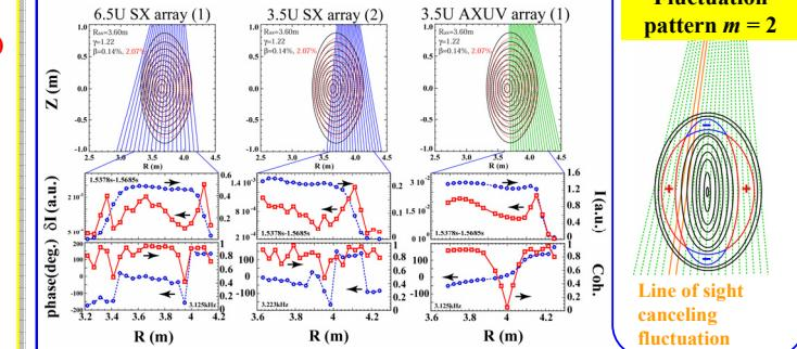
▪ Radial information of an edge MHD mode ( $m/n = 2/3$ ) observed by the SX and AXUV array on the vertically elongated sections of 6.5U and 3.5U ports is shown in this figures as a function of the major radius where the line sights of the SX and AXUV arrays intersect with the mid-plane of the LHD.
