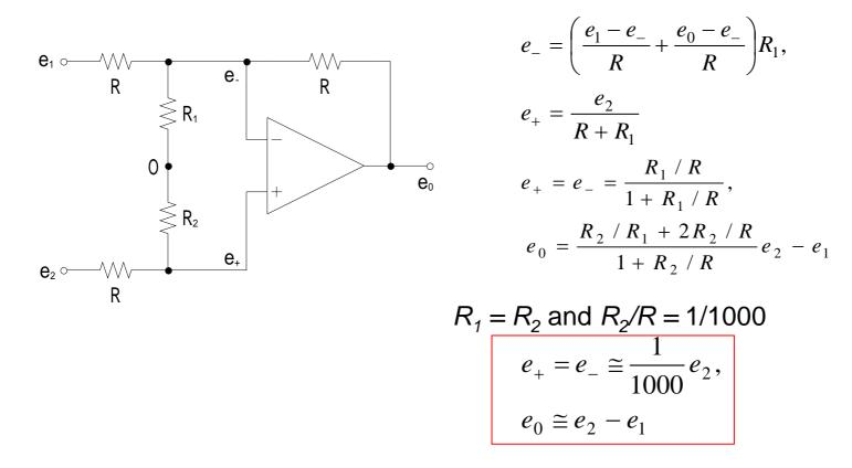
The input voltage of OP amp is  $\phi_s$  / 1000. The output voltage is a small voltage ( $e_2 - e_1$ ) of signal.
