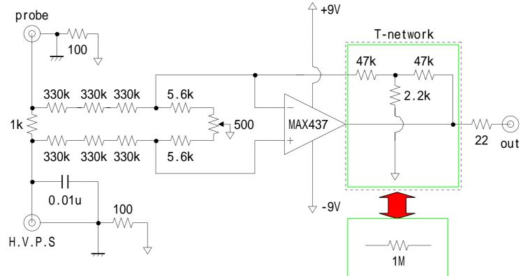
T-network can equivalently treat a small resistance as a large one in the feedback network.
