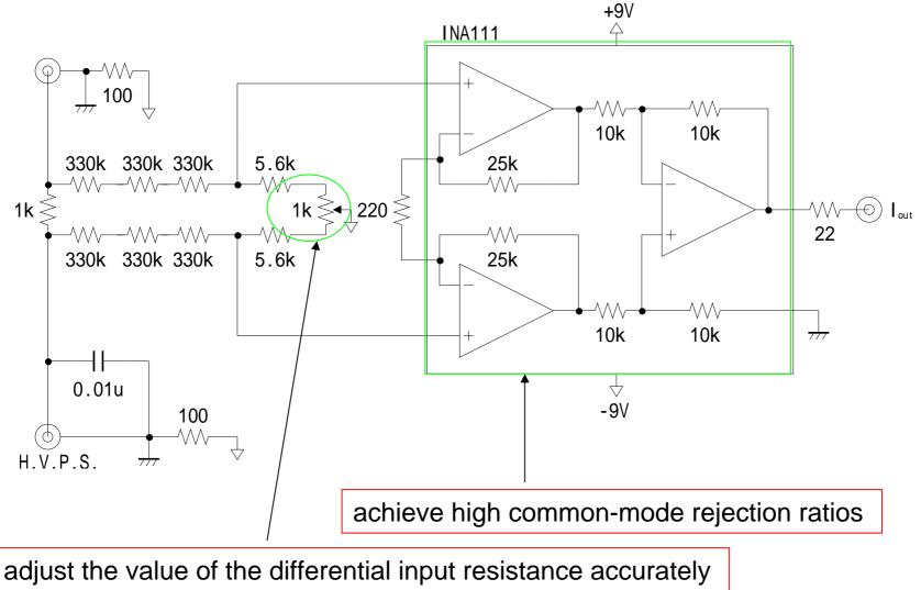
without using a single precise resistor
