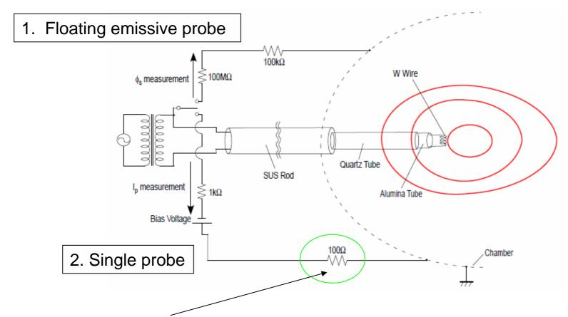
The reason why  $100\Omega$  is used is that the probing circuit suffered from substantial noise due to the ground loop on CHS. To alleviate the noise, the small resistance is installed in the probing circuit.
