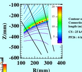
A clear lower boundary is found to exist irrespective of RF power level and coil current magnitude. Observed boundary fairly matches with the connection length contour plot.
