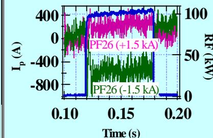
Plasma current direction is reversed when PF26 coil current direction is reversed.
