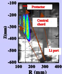
Plasma initially formed at the fundamental electron cyclotron resonance position
