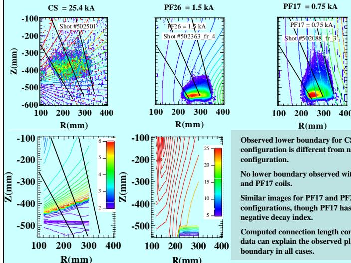
Observed lower boundary for CS configuration is different from null configuration.
