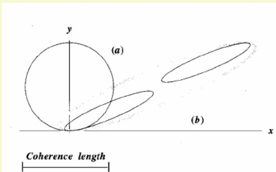
If the eddy is isolated it stretches into the shape indicated by the gray shaded curve. In turbulence, the eddy loses coherence in a coherence length, represented as a breakup into two eddies. The loss of coherence reduces the y scale relative to that of the reference eddy.
