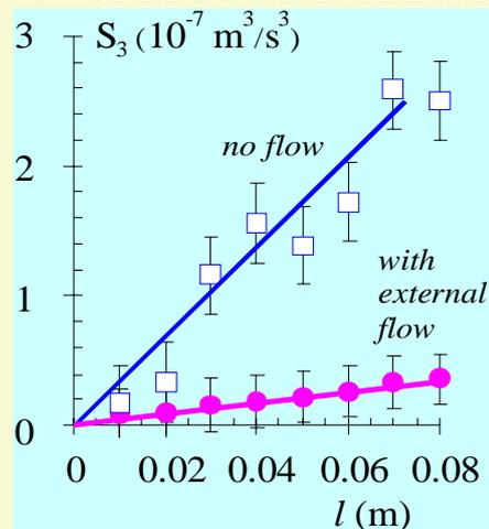
The energy flux through inertial range  $\varepsilon = -2/3 S_3(l)/l$
