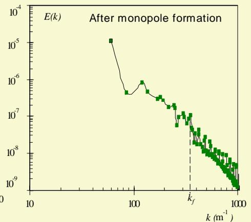
$k^{-3}$  power law is not due to the turbulent cascade, but rather due to coherent structures
