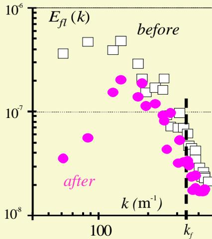
Shear suppression condition is satisfied in the middle of the energy inertial range
