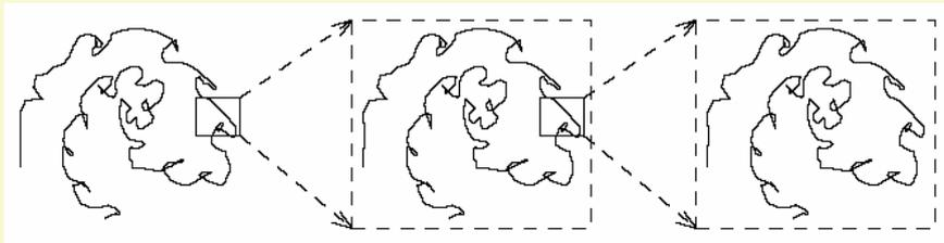
Self-similar cascade of eddies in a turbulent flow
