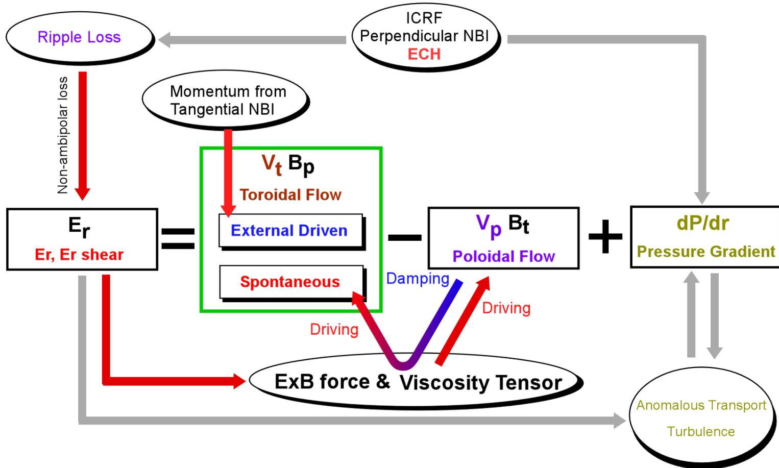
The radial electric field is determined by the non-ambipolar loss or pressure gradient and the coupling of ExB force and viscosity tensor drives spontaneous toroidal rotation.
