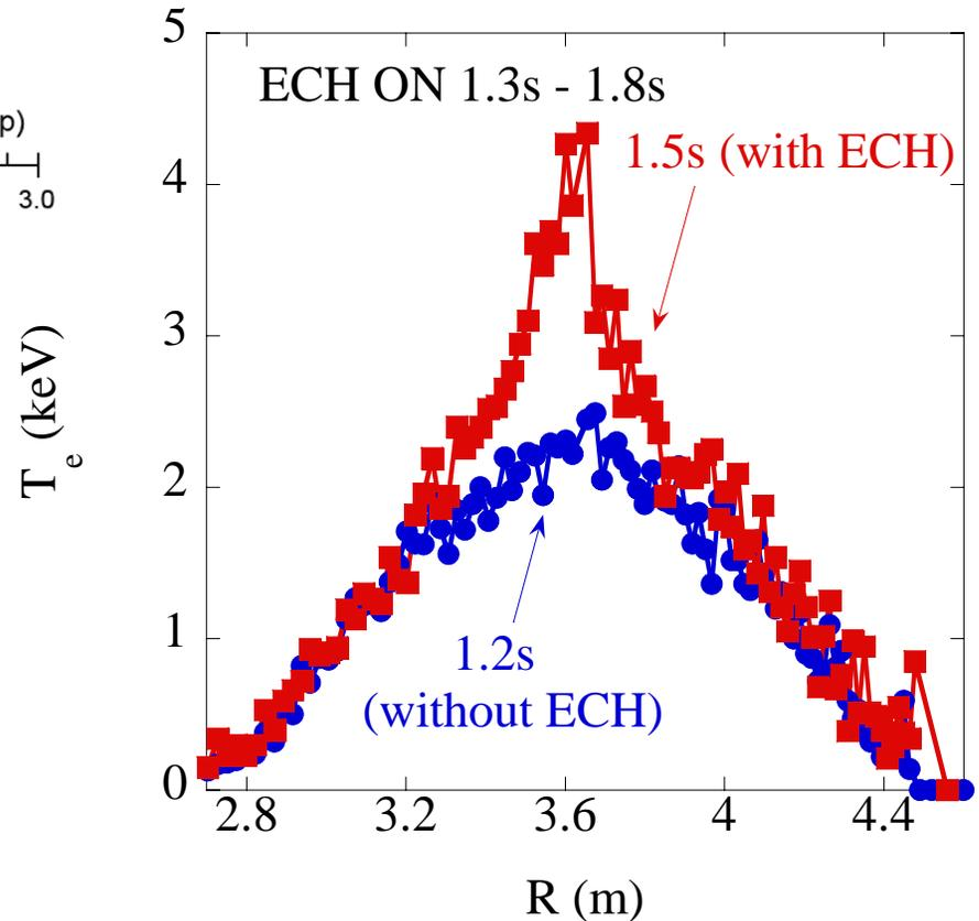
The CERC (Core Electron Root Confinement) profile is observed in the electron temperature, while the ion temperature has no significant change with the ECH.
