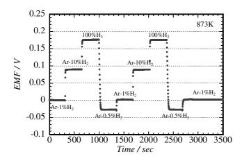
Fig. 1: The change of electro motive force (EMF) of Pd coated  $CaZr_{0.9}In_{0.1}O_{3-a}$  hydrogen sensor with the change of composition of gaseous environments.
