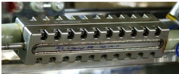
[The KSTAR lap joint of the SC bus-line]
