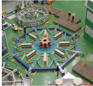
Jig System: Base Frame (2004. 01)
