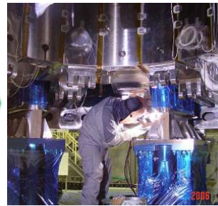
Assembly of VV Support
