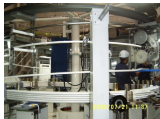
Turn Insulation Taping
