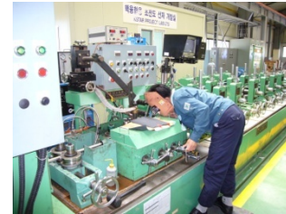
CICC Jack Welding
