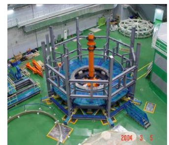
Jig System : Main Column (2004. 03)
