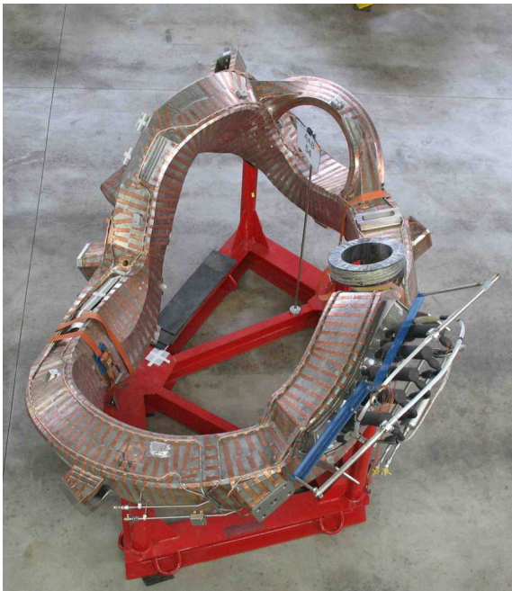
Fig.2 Non-planar coil AAB54 (type 4) on a transport frame. Clearly visible are the Copper stripes on the coil casing and the cooling tubes. In the lower right part of the picture, the header area with the five interlayer joints and the two superconductor tail ends can be seen.
