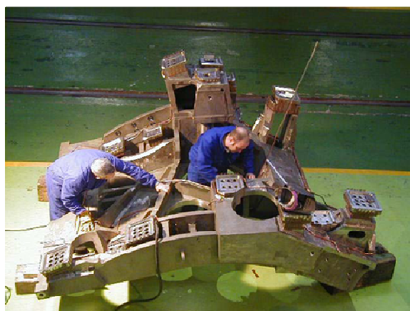
Fig.3 Final work on the first segment of the central support ring (1/10 of the full ring). The picture shows also the cast extensions and the contact surfaces for fixing the coils.
