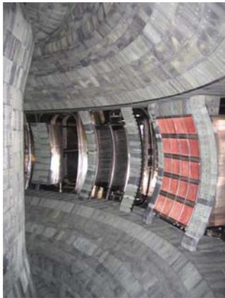
Fig.2 Picture of in-vessel together with the ICRF antenna and LHCD launcher
