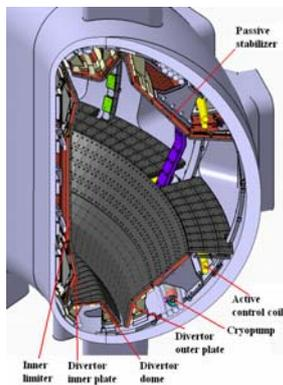
Fig.1 Elevation view of EAST in-vessel structure
