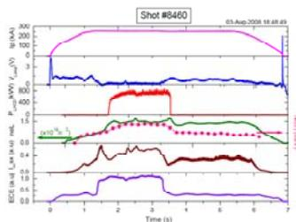
Fig.3 delivered 800kW LHCD power for nearly full non-inductive current drive
