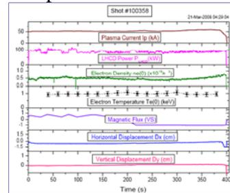
Fig.5 A long pulse discharge for 400s
