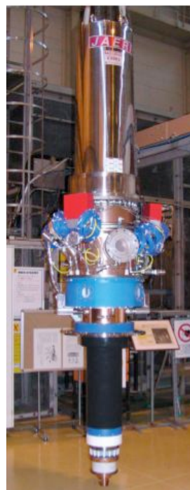
Fig.7: Picture of 170 GHz gyrotron. Oscillation mode is TE_{31,12} , and Gaussian beam output.
