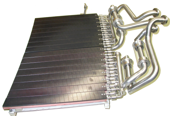
Fig.2 Two full scale prototype HHF target modules with dummy target elements, already mounted on adjustable frame.
