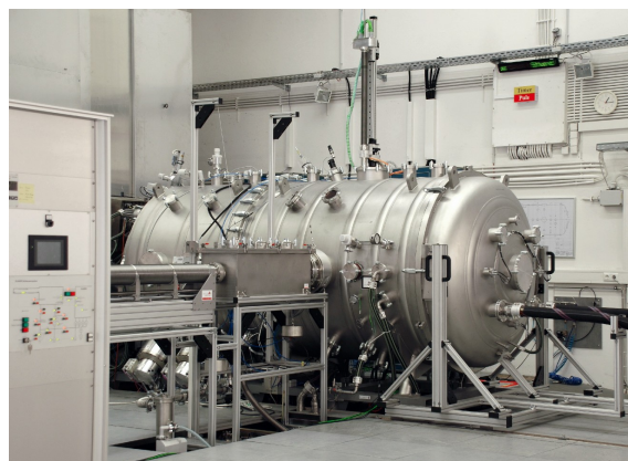
Fig.3 GLADIS HHF-test facility, with new designed vacuum lock
