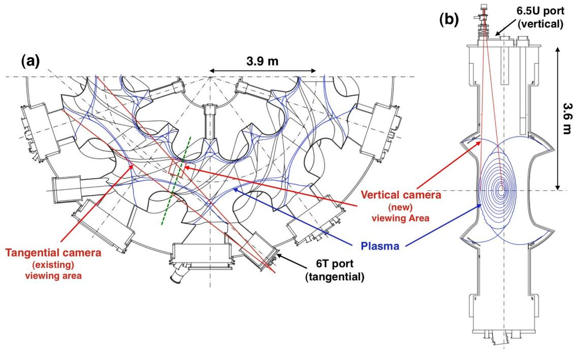
Fig. 1 Arrangement of the viewing areas of the existing and new soft X-ray CCD cameras. (a) Top view of horizontal cross section at the equatorial plane and (b) vertical cross section at the green broken line in (a) are drawn. The existing and new cameras have been installed in the tangential (6T) and the vertical (6.5L) viewports, respectively.
