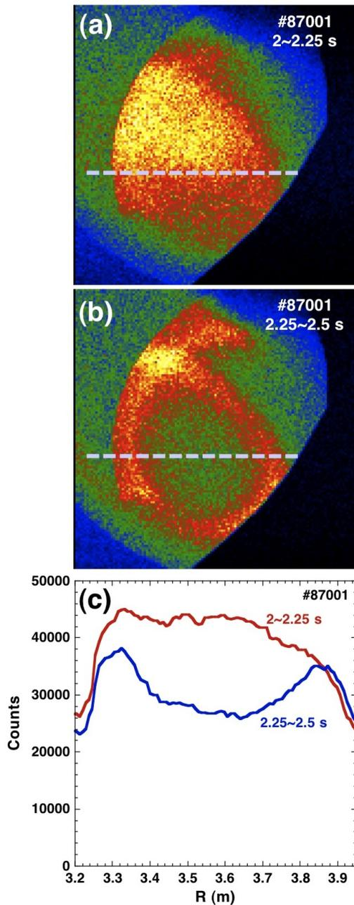
Fig. 2 An example of soft X-ray emissivity profile in a high ion temperature discharge with the formation of carbon impurity hole. The profile suddenly changes from (a) peaked one to (b) hollow one around 2.25 s when the formation of carbon impurity hole is observed in the charge exchange spectroscopy measurement. The change in the horizontal profile along the broken lines indicated in (a) and (b) is drawn in (c). The thickness of the Be filter is  $450 \mu\text{m}$ .
