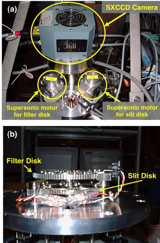
Fig. 4 Photographs of the installation of the new soft X-ray CCD camera system. (a) Installed CCD camera and two supersonic motors. (b) Filter and slit disks installed in front of the camera.
