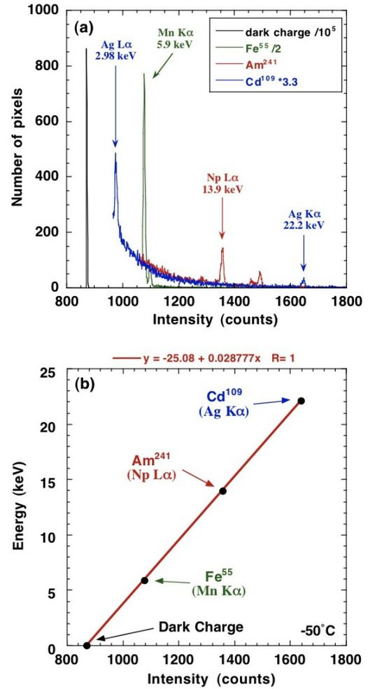
Fig. 3 Calibration of energy sensitivity and resolution of the new soft X-ray CCD camera. (a) Energy spectra obtained by several standard X-ray sources. (b) Plot of photon energy versus CCD count to obtain energy sensitivity from the slope.
