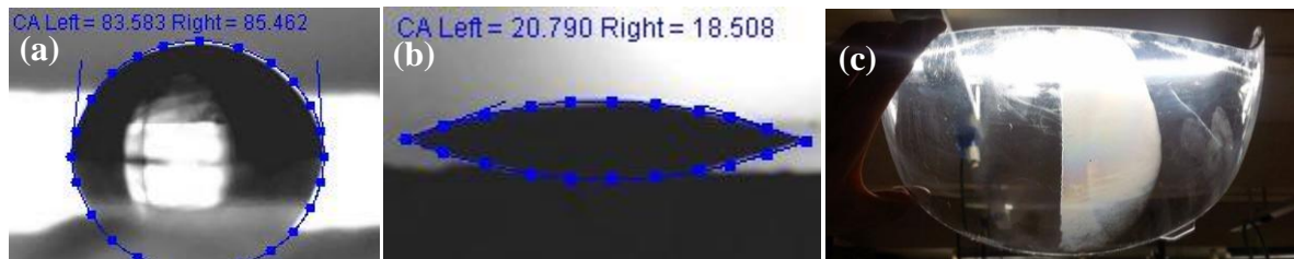
Figure 2. Contact angles of (a) untreated and (b) treated PMMA with nitrogen-argon flow rate ratio of 30:10 SCFH and a (c) photo of the visor after the condensation test.
