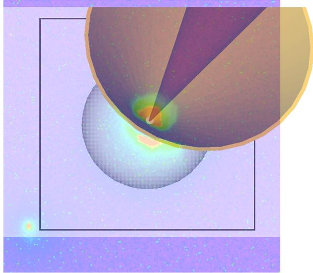
Figure 3. Time-integrated x-ray image of shell target with cone irradiated with Gekko-XII and LFEX lasers. Cartoon of the initial target is overlaid. Initial diameter of the shell is 500  $\mu\text{m}$ . The left bottom spot is a noise.
