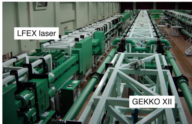
Figure 1. Gekko-XII laser system (right) for implosion of the fuel target, and LFEX laser beam line (left) for Fast Ignition heating.size.
