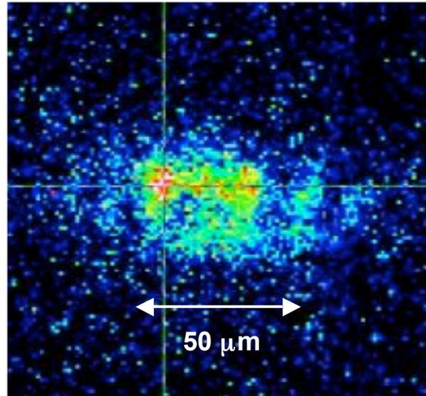
Figure 2. X-ray emission image of a Au plane target irradiated with LFEX beam, showing the LFEX focal spot size.
