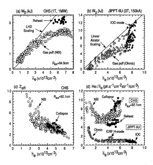
Fig. 2 (a) Stored energies in CHS (1T,  $R_{ax}$  = 94.9 cm) (b) Stored energies in JIPPT-IIU (c)  $Z_{eff}$  in CHS (d) Comparison of  $H_{\alpha}/\overline{n}_{e}$  between CHS and JIPPT-IIU as a function of line-averaged electron density  $\overline{n}_{e}$ . The  $H_{\alpha}/\overline{n}_{e}$  in ICRF L-mode plasma is 1.7 times as large as ICRF H-mode plasma with ELM.
