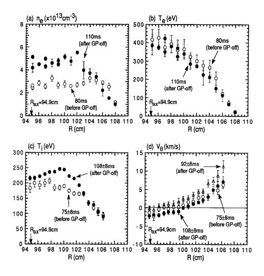
Fig. 3 Profiles of (a) electron density, (b) electron temperature, (c) ion temperature, and (d) poloidal rotation velocity in CHS at  $B_t = 1.5$  T,  $R_{ax} = 94.9$  cm and  $P_{NBI} = 1$  MW. In this case the  $W_p$  does not increase after switching off the gas puffing.
