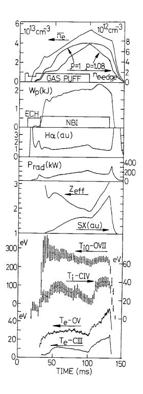
Fig. 1 Reheat mode of NBI plasmas in CHS ( $B_t$  = 1T,  $R_{ax}$  = 92.1 cm). The neutral beam is injected with a port–through power of 800 kW.
