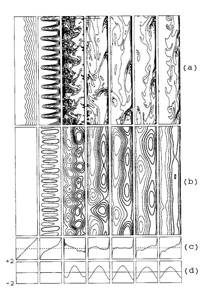
**FIGURE 4.** Snapshots of the contour lines for plasma density (a) and electrostatic potential (b) at the time moments  $\tau=4;5;6;8;10;15;20$  (from left to right) corresponding to the very first cycle of shear flow generation. Poloidally averaged profiles of plasma density (c) and poloidal flow velocity (d) are also shown (the case of  $g_B=7, \ \sigma_1=6$ ).
