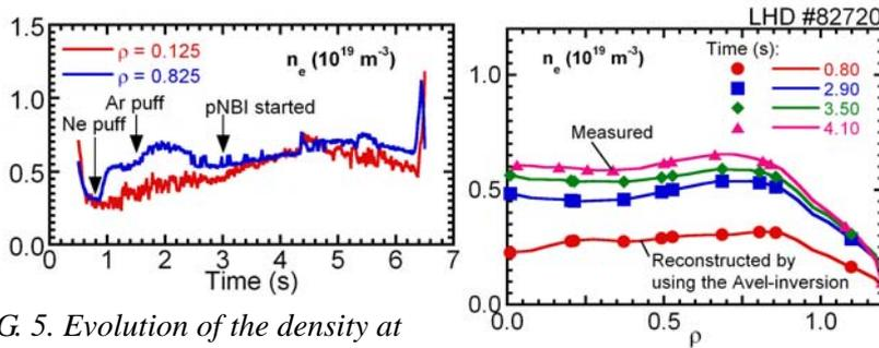
FIG. 5. Evolution of the density at different locations  $r=0.125$  and  $0.825$
