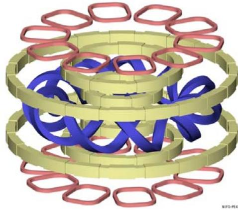
FIG. 5. Ten pairs of Resonant Magnetic Perturbation (RMP) coils (magenta).
