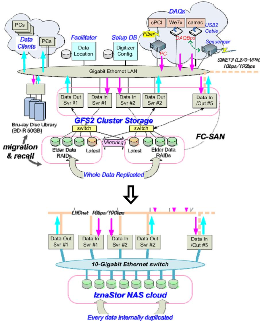
FIG. 3. Schematic view of the LABCOM DAQ and store system: The storage cluster had a mirrored structure on FibreChannel storage area network (FC-SAN) to store replicated files previously (left). They are replaced by distributed network attached storages (NAS) named “IznaStor” in 2010.
