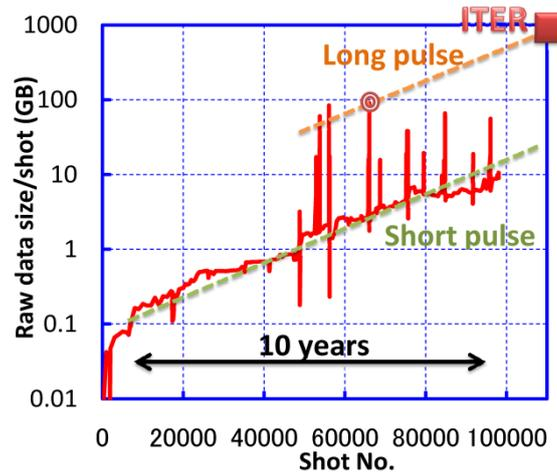
FIG. 1. Data growth in LHD: Each spike means the steady-state trial. A red double circle shows the world record of 90 GB.
