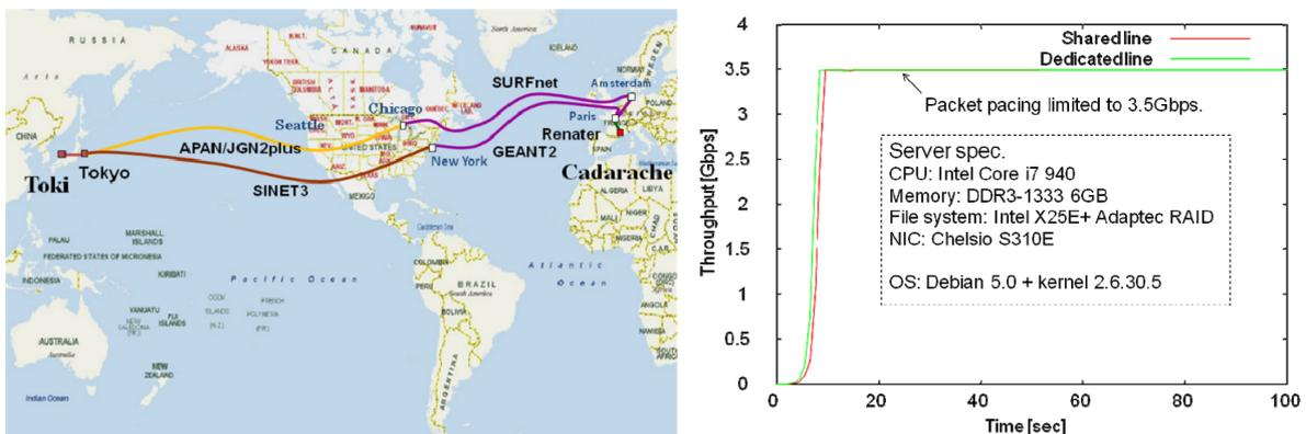
FIG. 5. Results of Japan-France bandwidth test: The fiber distance is about 15 000 km whose round-trip latency time is about 310 ms. Between 10 Gbps ports at both ends, the bandwidth was limited to 4 Gbps for the 10 Gbps shared backbone; SINET3, GEANT2, and Renater. The dedicated path through APAN/JGN2plus and SURFnet was also used.
