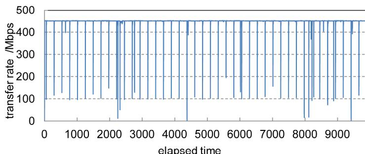
FIG. 6. Result of Japan-US bandwidth test between NIFS and GA, San Diego, CA: With the limited forwarding rate of 460 Mbps, very stable 451 Mbps throughput was obtained over 10 000 s. The comb-like drops are considered due to some periodical task awoken on the receiver computer.
