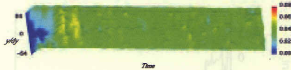
Figure 2: Spatiotemporal structure of off-plane electric field -E_z(t, y) for the narrow input window
