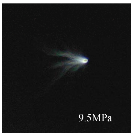
Figure 8. Photograph of the streamer discharge plasma at pressure of 9.5MPa and at temperature of 37°C.
