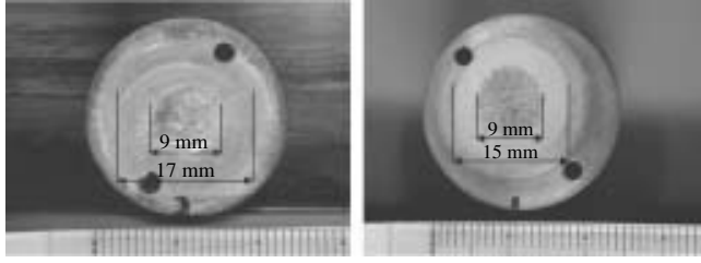
Figure 6: Damage patterns in the upstream and downstream sides of the cusp. The outer radius of the damage was decreased at the downstream side of the cusp field.
