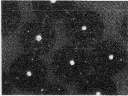
Fig.1. Spherical copper powder particles of 120μm in diameter
