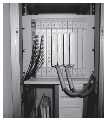
Fig. 2 New data acquisition system for the real-time judgment of normal-transitions.
