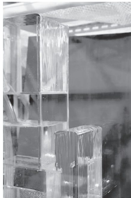
Fig. 3 Flow visualization by using water as a coolant and you can see the stable water falling film flow on the vertical wall of the test section
