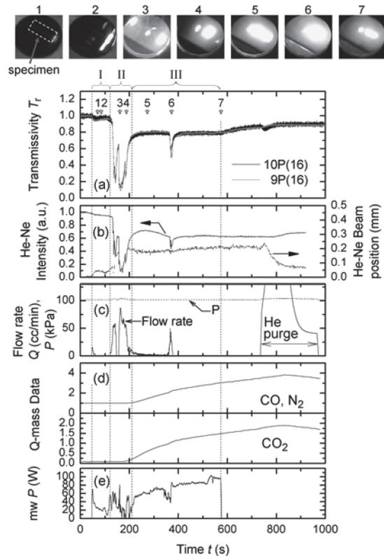
Fig. 2. Various time evolutions measured during the microwave carbothermic reduction of magnetite. CO<sub>2</sub> laser transmissivities in (a). Intensity of the transmitted He-Ne laser and its beam position in (b). Flow rate of exhaust gas and gas pressure in (c). Component intensity in CO and CO<sub>2</sub> measured by Q-mass in (d). Net absorbed power into the cavity in (e).
