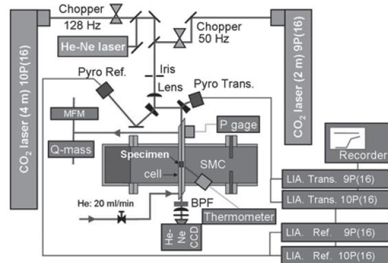
Fig. 1. Experimental setup of the microwave heating in the single mode cavity (SMC) and the LAS diagnostics system.
