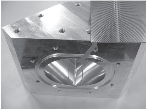
Fig. 3 Corrugated miter bend
