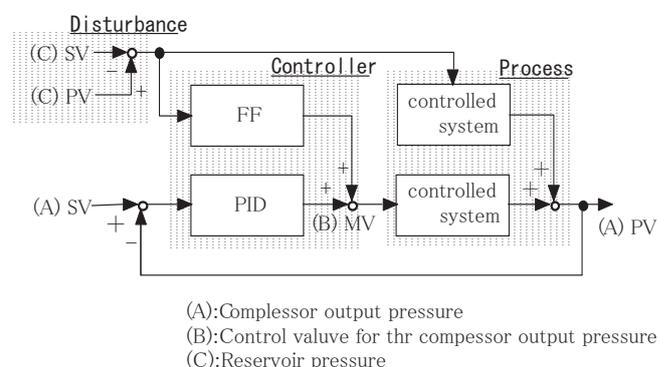
Fig.24 Block diagram of advanced control algorithm
