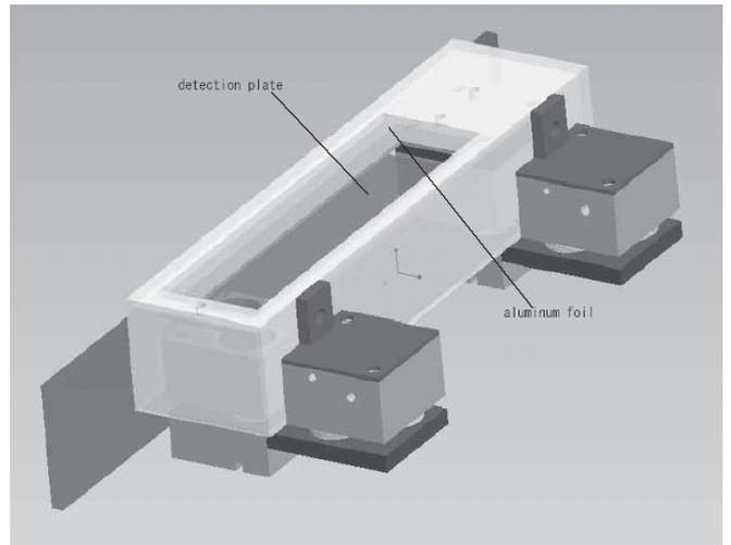
Fig.18 First beam monitor remodeling in vacuum container.
