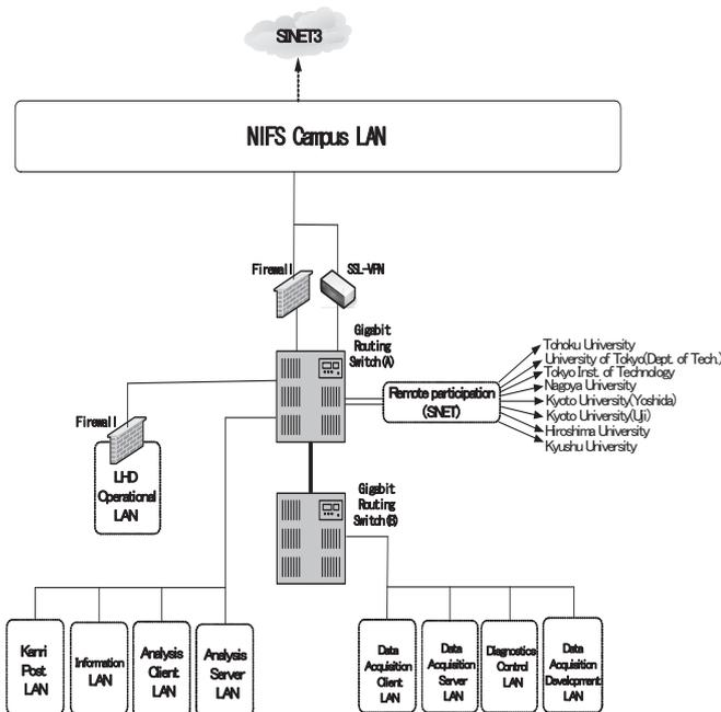
Fig. 27 Block diagram of LHD-LAN
