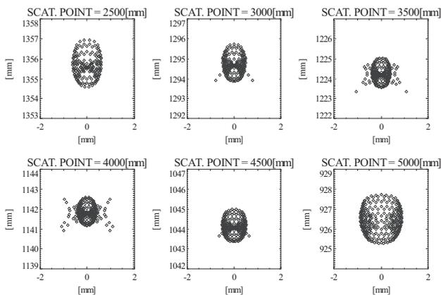
Fig.16 The spot diagram focused with the spherical mirror.
