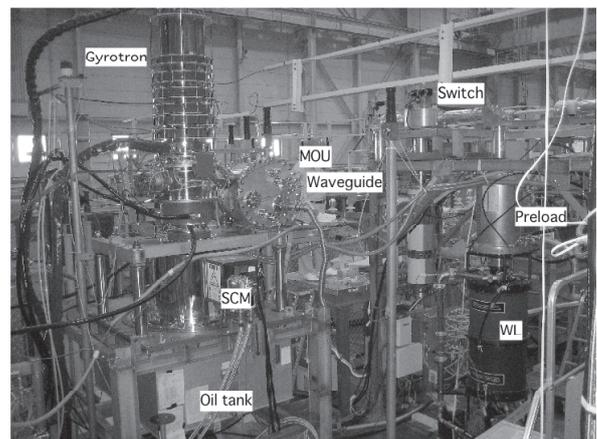
Fig. 10 Transmission line from a new gyrotron to dummy load (Water Load).
