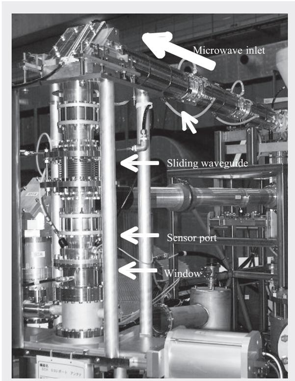
Fig.11. Improvement of 3.5inch diameter waveguide components on LHD.
