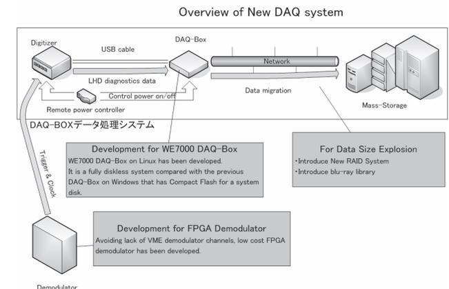
Fig. 22 Change to new DAQ system with DAQ-Box
