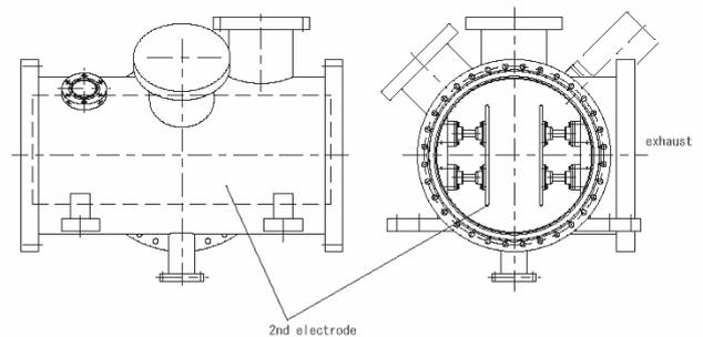
Fig.19 2<sup>nd</sup> electrode installation design of exhaust chamber
