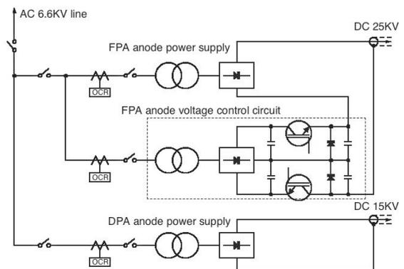
Fig. 12 FPA anode voltage control circuit
