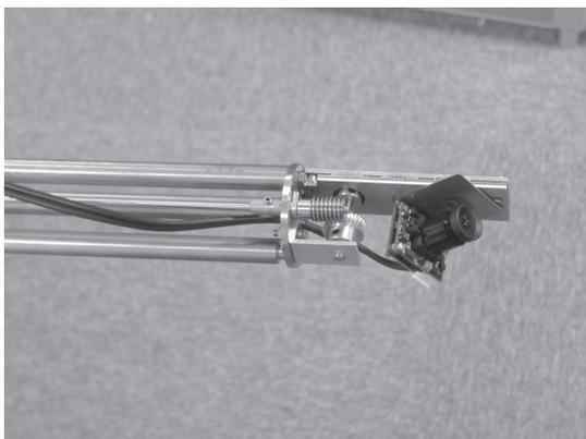
Fig. 29 Drive mechanism of the CCD-camera
