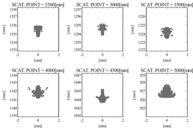
Fig.17 Spot diagram focused with the aspherical mirror.
