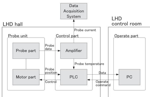
Fig. 14 Diagram of remote control system for probe
