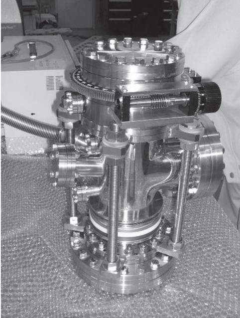
Fig. 20 Snap shot of the vacuum leak test of the ARMS in the Plasma Diagnostic Laboratories
