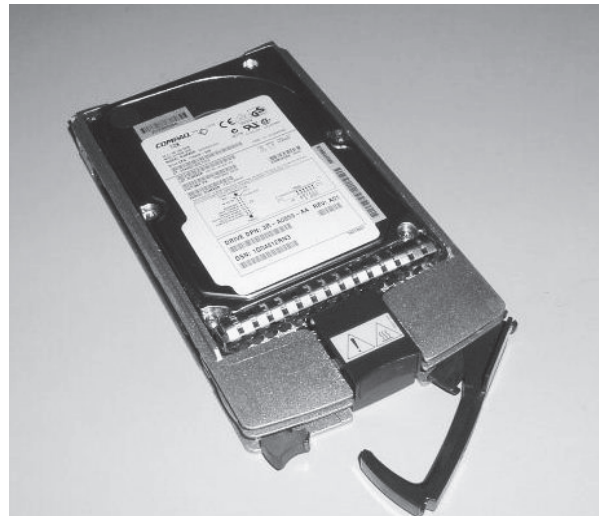
Fig.1. The movable disk unit that is installed the DS20E Tru64/VMS data analysis server.
