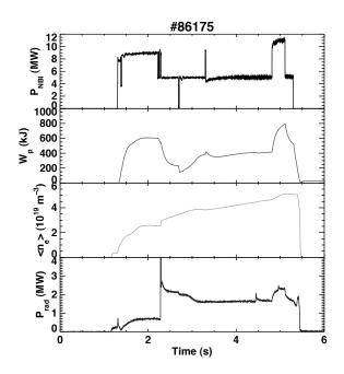
Fig. 1: Time sequences of NBI heating power  $(P_{NBI})$ , stored energy  $(W_p)$ , line averaged electron density  $(\langle n_e \rangle)$  and total radiation power  $(P_{rad})$  in a LHD discharge with a tungsten pellet injection at 2.3 s.
