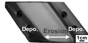
Fig. 1. After exposed VPS-W tile using at the inner position of the helical divertor.
