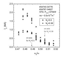
Fig. 2 Measured current as a function of the magnetic field strength at  $N_{\parallel}\!\!=\!\!0$  and  $N_{\parallel}\!\!=\!\!0.38.$
