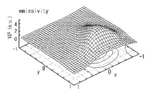
Fig. 2 Plasma image which was reconstructed by combining 12 basis functions as a result of training for numerically-simulated projection data of a phantom.
