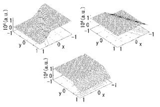
Fig. 1 Three basis functions which contribute to forming the edge of the semi-tangential cross section of LHD: the image region to [-1, 1] in both the *x* and *y* directions.
