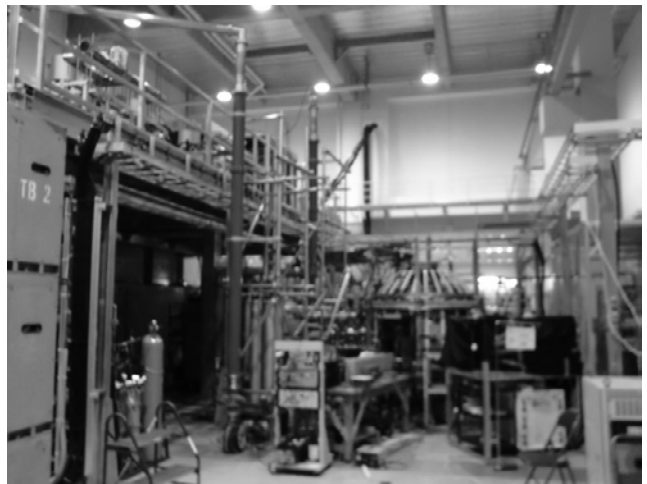
Fig. 1. Photograph showing the coaxial transmission lines to deliver RF power from 200 MHz transmitters installed on the mezzanine level to the two-strap loop antenna installed inside the TST-2 vacuum vessel.
