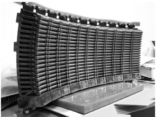
Fig. 2. The TST-2 eleven-element combline antenna. RF power is fed to the antenna array from one end, propagates to adjacent elements by mutual inductance, and the left over power not radiated into the plasma exits from the other end of the antenna array.
