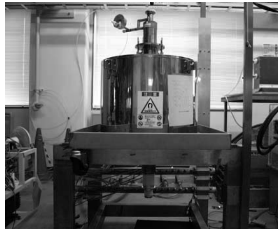
Fig. 1. Sealed-off gyrotron mounted on the 8 T superconducting magnet. This picture was taken before setup of the gun coils.
