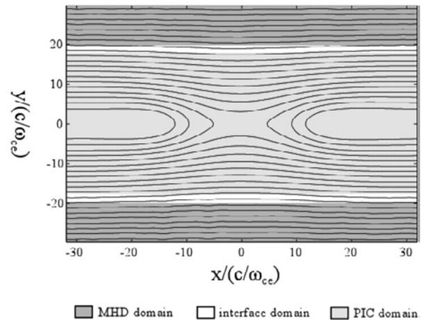
Fig. 2: Magnetic field lines of force in multi-hierarchy simulation.
