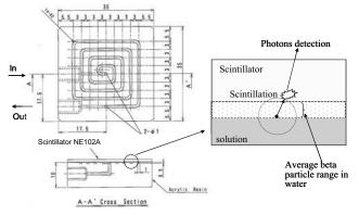
Fig. 1. An equipment of tritiated water flow presumed to be collected from air sampling system and detection image by plastic scintillator.
