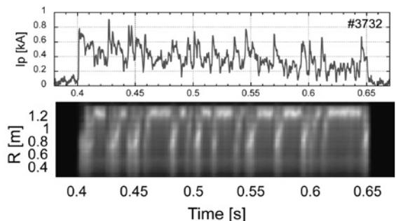
Fig. 4 Time evolution of  $I_p$  and contour plot in radial direction of  $H\alpha$  emission captured by medium-speed camera.
