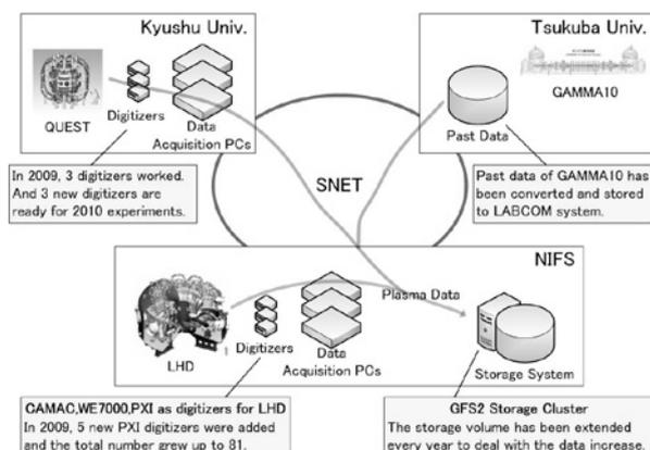
Fig. 23 Overview of the LHD Data Acquisition System.
