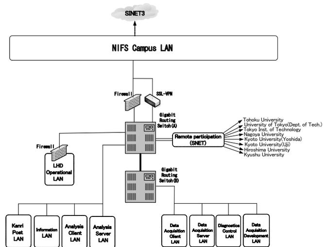
Fig.29 The schematic structure of the new LHD-LAN
