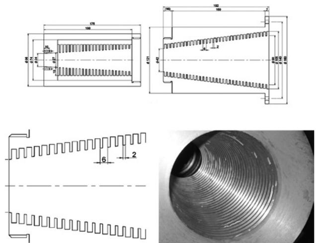
Fig.1 Corrugated Horn Antenna.
