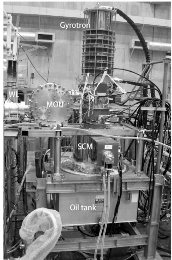
Fig.10 A new 77GHz/1.5MW gyrotron system
