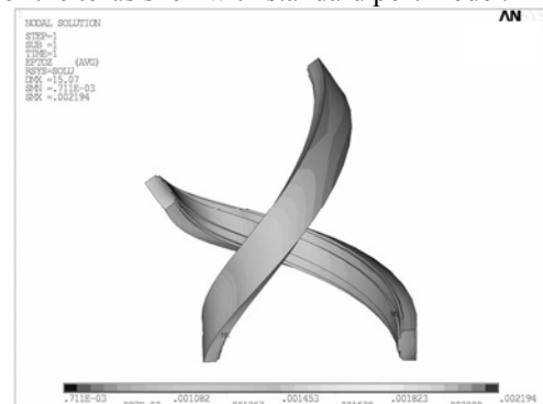
Fig. 4. The hoop strain distribution in the helical coil for the quasi-three-dimensional model.
