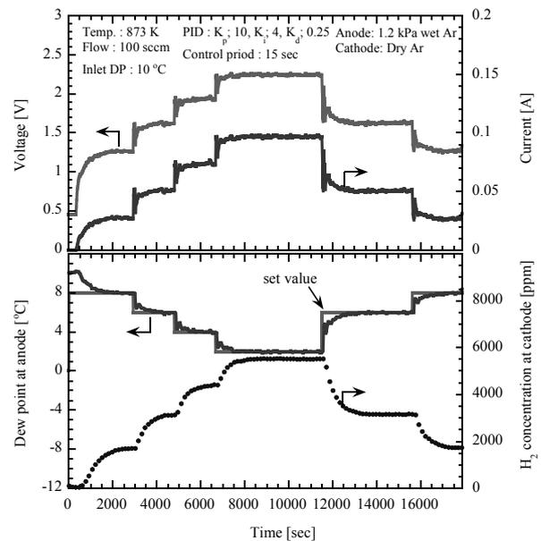
Fig. 2. Variations of voltage, applied current, dew point at the anode, and hydrogen concentration at the cathode under the feedback control.
