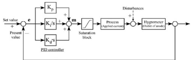
Fig. 1. A schematic flow diagram of PID feedback control system.
