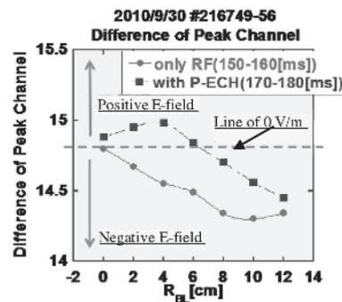
FIG. 1 The preliminary results of the radial profile of the radial electric field with and without P-ECHR
