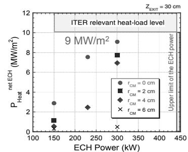
FIG. 2 The dependence of heat flux density near the mirror throat on the ECRH power.
