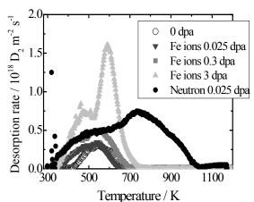
Fig. 1 Thermal desorption spectra of deuterium from W damaged by neutron irradiation and Fe ion implantation after exposure to deuterium plasma at  $473 \text{ K up to} \sim 10^{26} \text{ D m}^{-2}$ .
