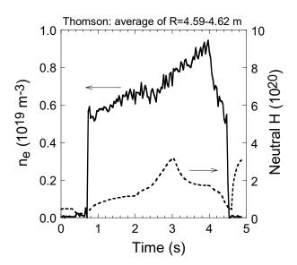
Fig. 2 Time evolution of edge plasma density and neutral hydrogen contents of the vacuum region in high density plasma. ECH power was applied to the NBI plasma from 2 s to 3 s.
