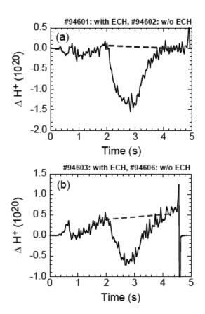
Fig.1 Time evolution of difference in total number of hydrogen ions in the plasma between discharges with and without ECH. (a)Low density plasma and (b) high density plasma. ECH power was applied to the NBI plasma from 2 s to 3 s.
